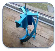
A self starting Vertical Axial Wind Turbine intended for domestic wind harvesting, but could be scaled to any application.
